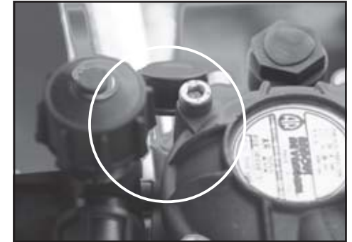
Check pump oil level regularly.
