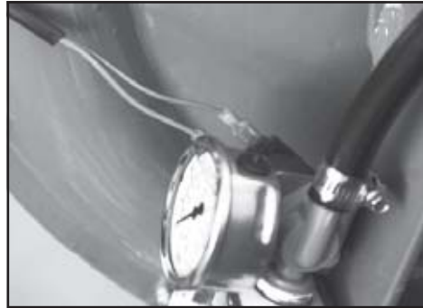
Connect brown & red wires to the solenoid.
