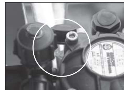
Check pump oil level regularly.
