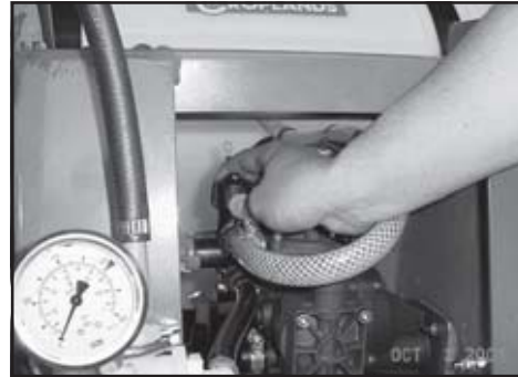
Use the manual control knob to adjust pressure.
