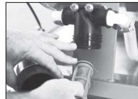
Ensure both O-rings are in place & in good order.
