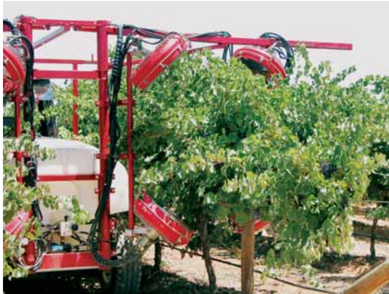
Photo shows heads set in sprawling canopy
