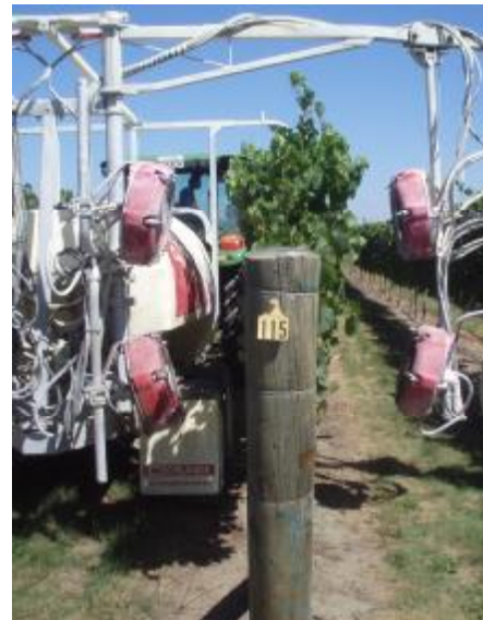
Figure 6: Showing the sprayer with heads configured for achieving the coverage shown in Figures 4 and 5.
