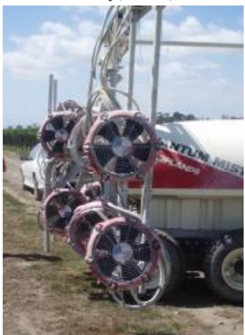
Figure 2 The QM380 heads on a three row sprayer in Marlborough
