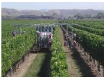
Figure 1 A three row Quantum Mist™ sprayer with QM380 heads on a 2.4m row merlot block in Hawkes Bay (Feb 2008).
