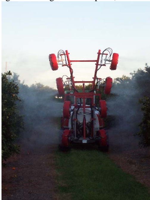
Pictured at left: Quantum Mist™ eight-head tower sprayer working in citrus.
